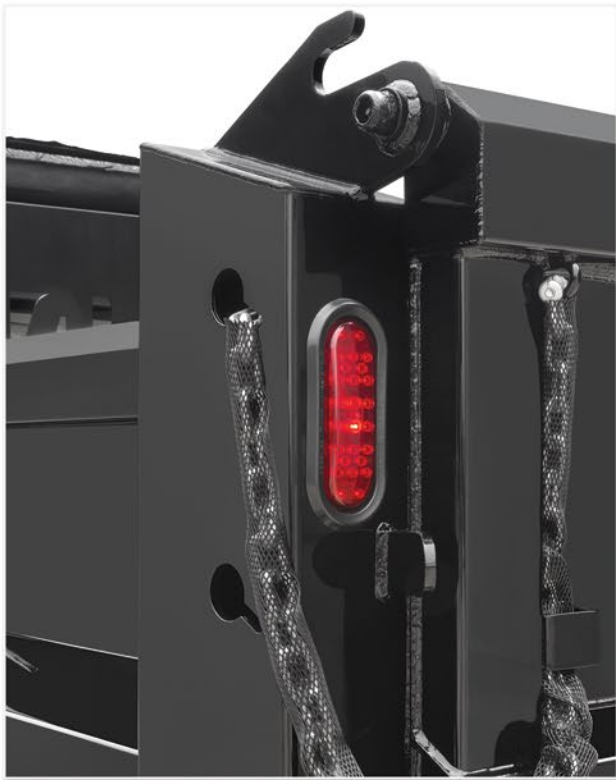
Heavy-duty mesh chain covers and redundant recessed lighting enhance safety.
