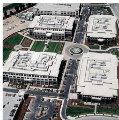
▲ This impressive complex in northern California is protected by a Paradiene 20/30 System installed over Siplast Lightweight Insulating Concrete.
