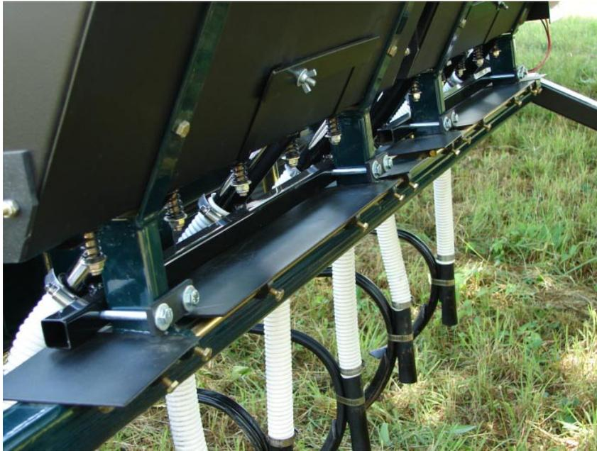
**There are (2) Sets of dispensing bars that affix to the “Y” bracket mount under each seeder, each dispensing bar has (3) metal tubes that join the flex tube and then is secured to the rear of the “S” tine so the seed falls directly into the furrow**
