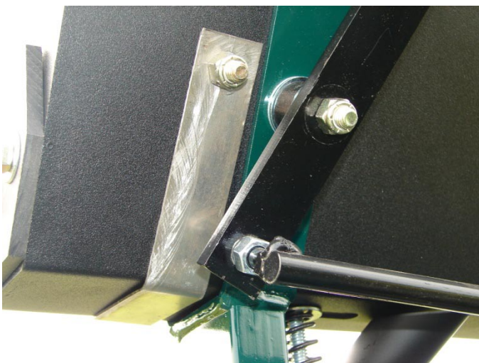
2 "SEAL OFF" SHEILDS ARE USED ON THE HUNTER 400 TO SEAL OFF THE TWO OUTER HOLES OF THE 30" SEED BOX TO INSURE NO LOSS OF SEED WHEN USING THE 4 ROW PLANTING SYSTEM.
