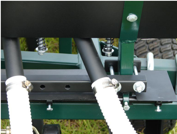
1 SET OF LOCATION HOLES ARE FOR MOUNTING THE DISPENSING TO THE UNIT; INNER HOLES DEPICT THE DESPENSING BAR MOUNTED ONTO THE HUNTER 300, THE OUTER HOLES DEPICT THE DESPENSING BAR MOUNTED ONTO THE HUNTER 400. (AS SHOWN ABOVE ON 400)
