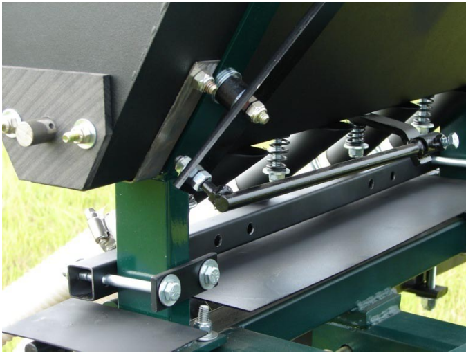
BACKING PLATES COUPLED WITH THE 5/16" X 4" HEX BOLTS ARE FOR SECURING THE DESPENSING BAR TO THE "Y" SEED BOX BRACKET.
