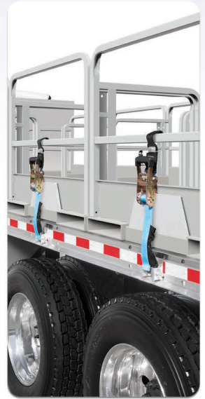
Tombstone and cargo straps secure bottled gas pallets to body
