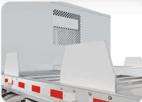
Tombstone sizes and locations can vary to accommodate bottled gas pallets
