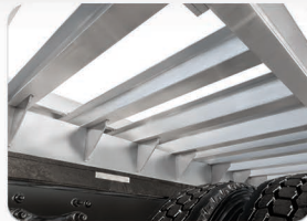
4" Aluminum I-beam crossmembers; 6" structural aluminum channel longrails
