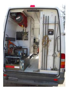
Mobile video units carry all the equipment necessary to conduct a video inspection. Once the camera equipment has been staged in the pipe, a reel containing 1,500' of single conductor cable enables the operator to remotely control the camera's functions and pace during the inspection and transmit video and data to the on-board computer.
