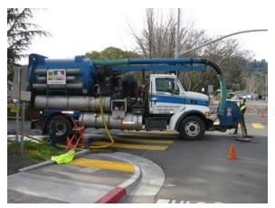
Combination machines containing both pipe cleaning and vacuuming capabilities produce 2,000-2,400 psi at 60 to 80 gpm. On-board water tanks hold 1,500 gallons for pipe cleaning procedures and a ten yard debris tank retains material removed from the pipe.
