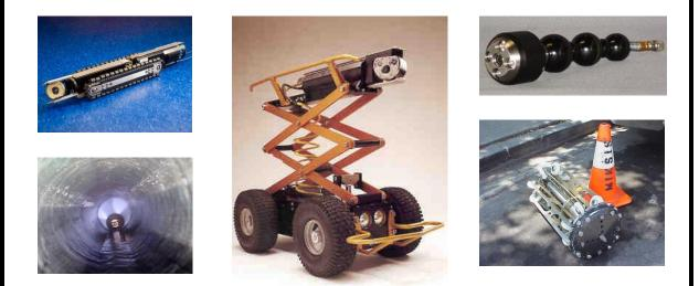
The results of the pipeline video inspection are produced in a digital format submitted in DVD format or on a hard drive. Written reports accompany the video for each pipe segment inspected. Any faults detected in the pipe are noted along with the their footage location. Pipe assessment is in accordance with PACP standards.
