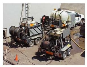
Harben jetters produce 4,000 psi at 12 gpm with a 500 gallon water tank. These units are effective in cleaning pipe from 2" to 8" in diameter.
