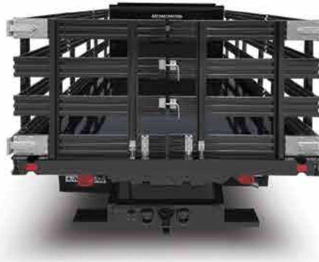
Morgan's innovative swing rack design eliminates the need to lift and remove heavy racks in order to load or unload. Heavy duty hinges allow each gate to swing a full 270-degrees, where they can be secured to the siderails for easy and unencumbered loading and unloading.
