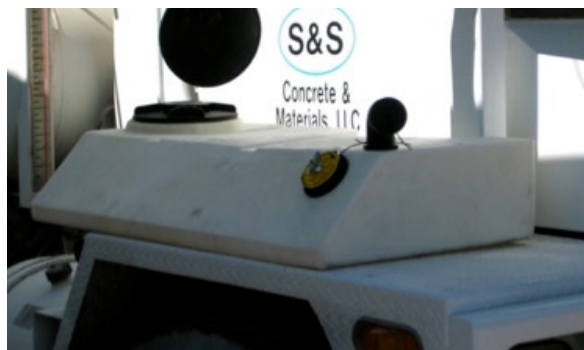
FRONT DISCHARGE TANK
