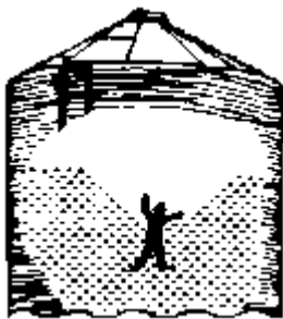
Figure 5. Flowing Material Traps and Suffocates
