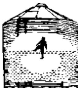
Figure 7. Crusted Material Collapses and Suffocates
