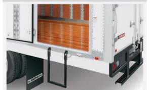
Strategically placed side-doors, steps and grab handles are ergonomically designed to enhance safe and convenient access to the cargo area.
