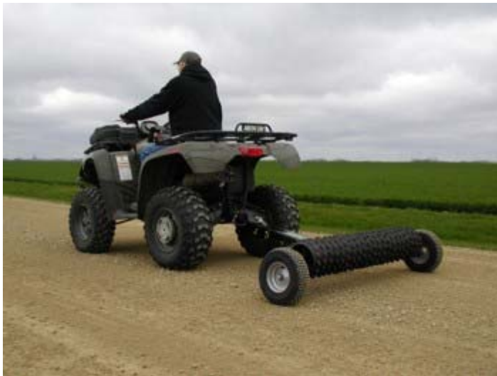
The Models TP2148 and TP3272 can have the Wheel Kit option added. This allows the TP Cultipackers to be flipped over for easy transport behind ATVs and UTVs.
