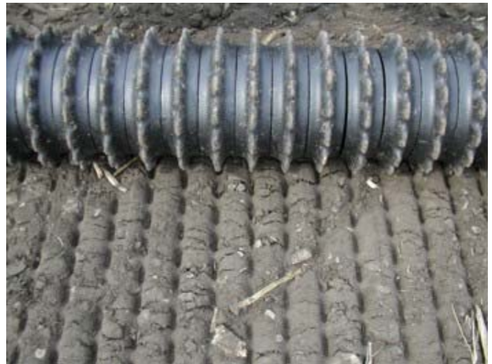
The TP Cultipackers will also leave dimples in the ground. These dimples will retain moisture and provide an excellent environment for rapid, dependable germination.
