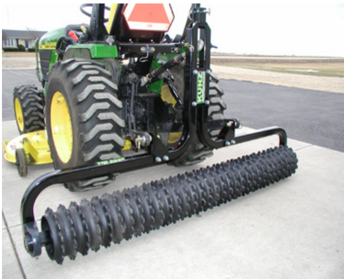
The Models TP2148 and TP3272 can be mounted to the back of a tractor with the optional 3-Point Kit.
