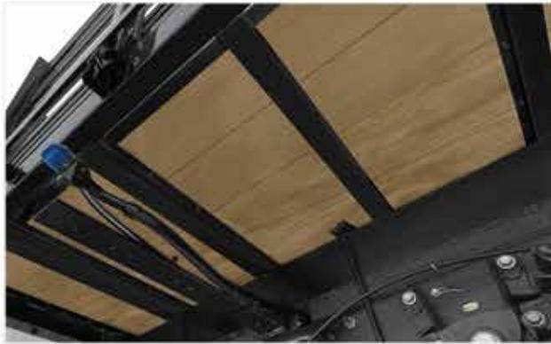
Three-inch I-beam frame construction delivers superior strength and durability. Positioning crossmembers 16 inches on-center reduces weight for better fuel efficiency.
