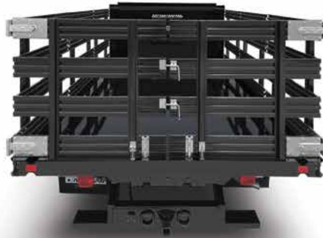
Morgan's innovative swing rack design eliminates the need to lift and remove heavy racks in order to load or unload. Heavy duty hinges allow each gate to swing a full 270-degrees, where they can be secured to the siderails for easy and unencumbered loading and unloading.
