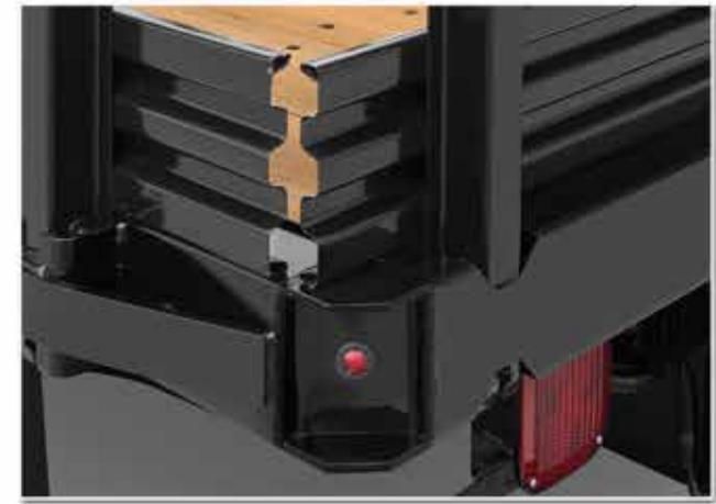
Deep pocket design provides solid seating of upright stake racks; making it easy to secure your load during transport, and remove racks for loading and unloading.
