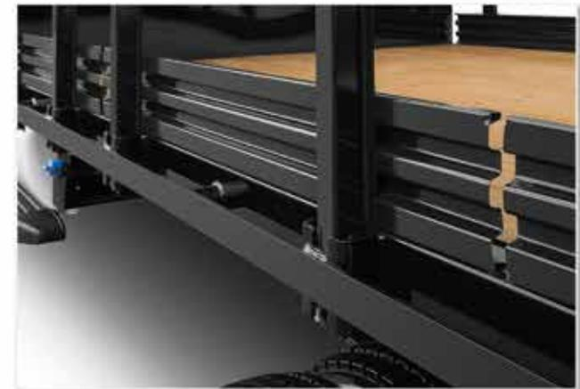
A standard, heavy-duty rub-rail helps to protect the flatbed frame and side rail pockets from minor impacts.
