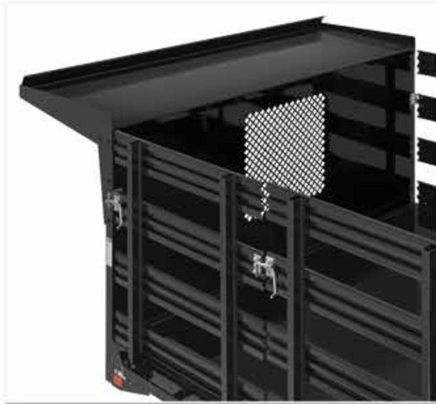
A heavy-duty steel cab extension helps to protect the cab against damage caused by dirt, debris or movement of bulk materials during loading and unloading.
