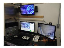
The launch system camera can be remotely rotated by the operator for easy insertion into the lateral with a range of up to 100'. Assessments regarding the condition of the sewer lateral are compliant with NASSCO LACP.
