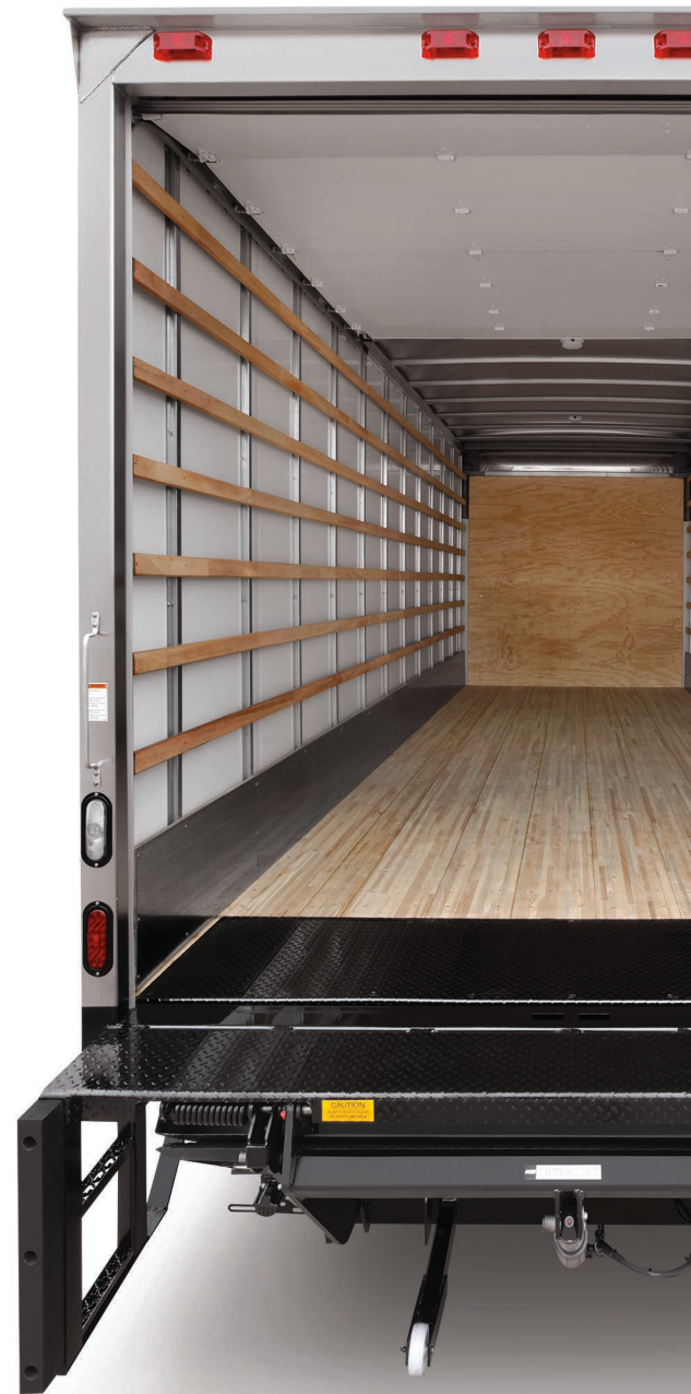
Cargo Interior Shown with Tie Slats and Steel Scuff
