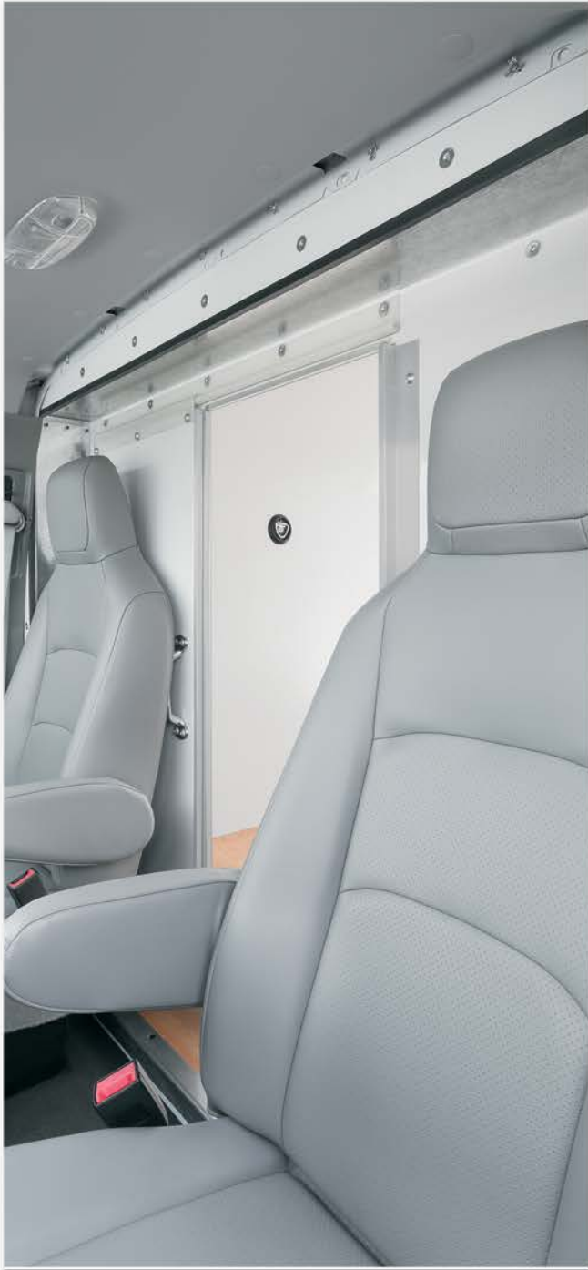
An option for a cab access door with a standard recessed bulkhead that provides more room in the cab and easier positioning of the seat.
