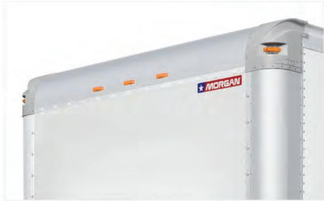
Morgan innovation changed the van body industry when they produced a body that is aerodynamic in design, and features patented poly-tuff corners, and a reinforced front-end.
