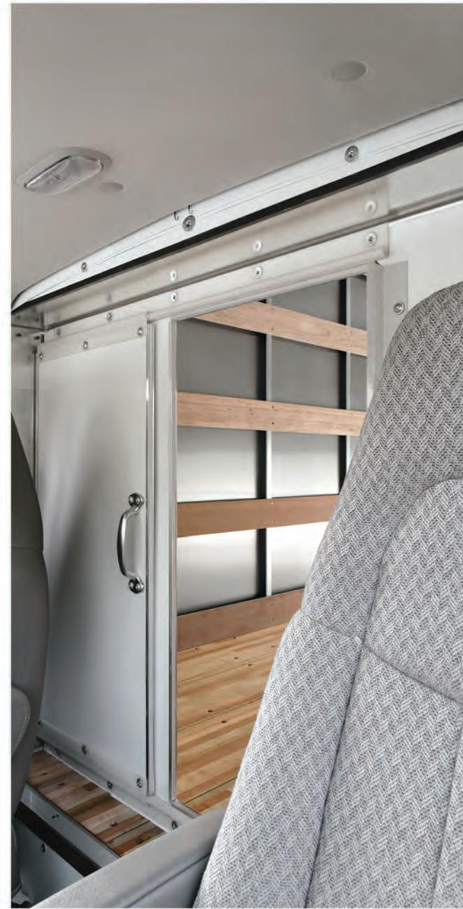
Morgan's Parcel Van cab configuration helps to reduce driver exposure to the elements (and traffic) by providing quick and easy access to the cargo area from the cab.
