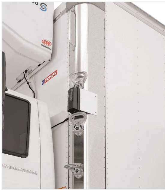
Strategically placed grab handles and a variety of service step configurations provide easy access to the service platform, and lend to a safer work environment.
