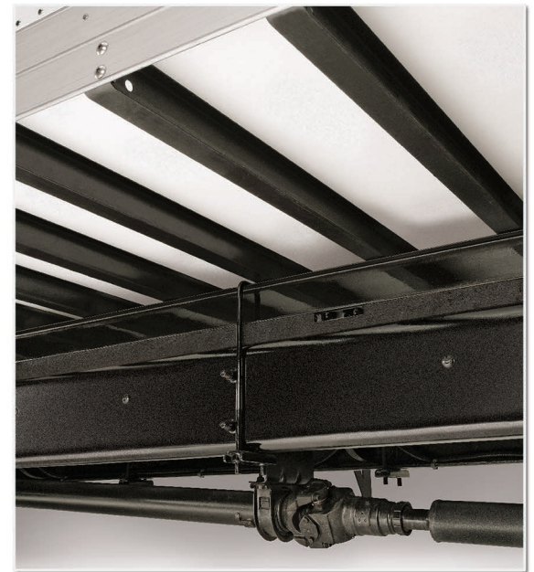
Refrigerated Body's floor is fully insulated using Morgan's poured-in-place polyurethane foam process to ensure consistent density and equal insulation across the entire floor.
