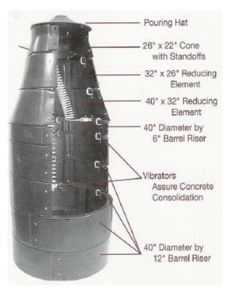
A cast-in-place concrete liner designed to rehabilitate existing manholes. Modular forms are constructed inside the manhole structure. A monolithic concrete pour between the form and the existing wall creates a solid manhole surface. The procedure is quick and requires no interruption of flow.
